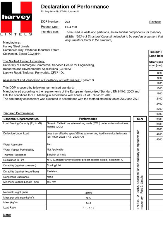
TableA1: Load bearing capacity Clear Opening SWL UDL (kN) span (mm) 600 191 900 191 1200 191 1500 191 1800 191 2100 191 2400 191 2700 191 3000 191 hEN 3300 174 3600 160 3900 148 for 4200 138 : 2012, Specification for ancillary components Part 2: Lintels 4500 129 845 - 2 : masonary -
